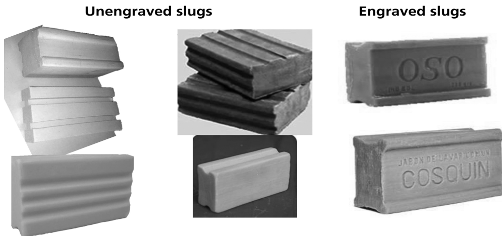
Figure 9.10 Unengraved and engraved extruded slug shapes.
