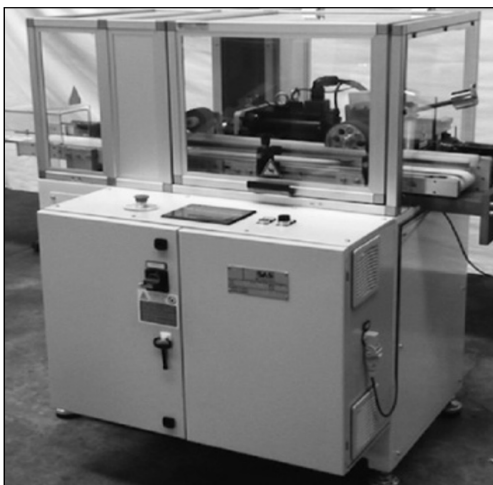
Figure 8.33 SAS Easycut two-blade electronic cutter. Source: SAS.
