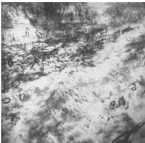
Figure 2.10 Characteristic optical pattern of a hexagonal liquid crystal viewed through a microscope fitted with cross polarizers.
